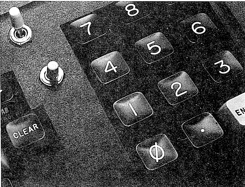
Photo 3. The period/comma switch mounted on the CPU. (The upper switch is an upper/lower-case switch.)
